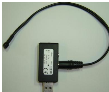
xEC-IR shown with the supplied External IR receiver eye.
