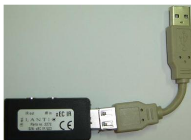
xEC-IR shown with optional USB extension cable using the built-in IR receiver.
